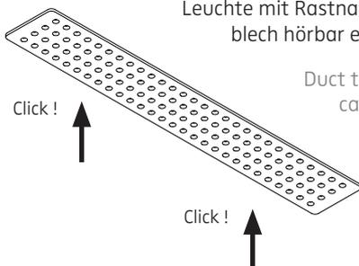
Duct the cables carefully into cavity, click the luminaire onto mounting plate by means of the snap-in noses.
